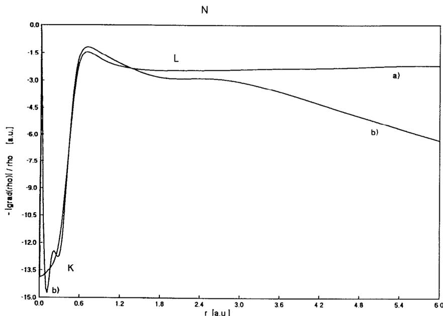
FIG. 8.  $-|\nabla\rho|/\rho$  for the HF calculation of nitrogen. The all electron calculations were realized with (a) the Lie/Clementi (Ref. 22) and (b) the STO-3G (Refs. 20 and 21) basis set. The shells are marked by capital letters.
