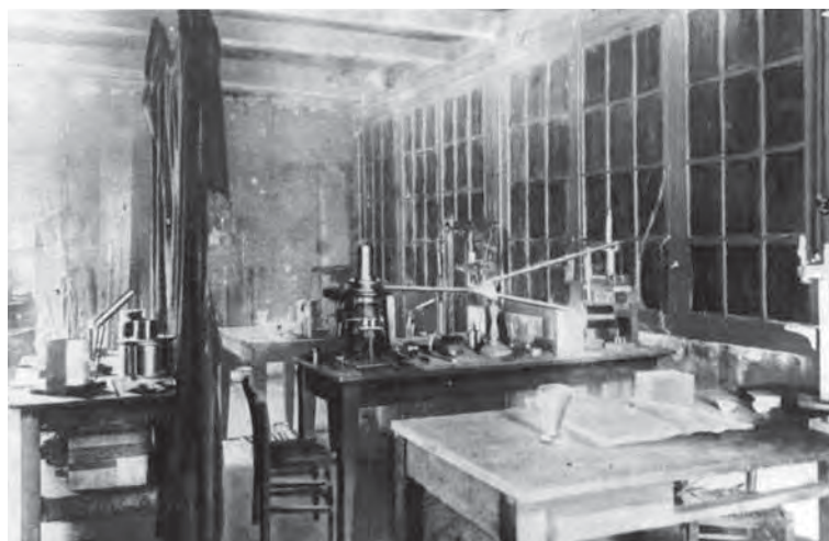
The “Curie Laboratory”: left, chemistry bench; right, ionization chamber and electrometer.
